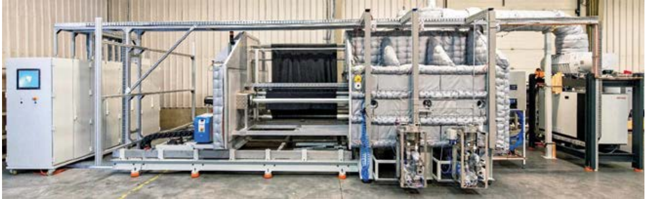
FIGURE 1: Europlasma roll-to-roll vacuum plasma coater CD1800/800 Nanofics.
