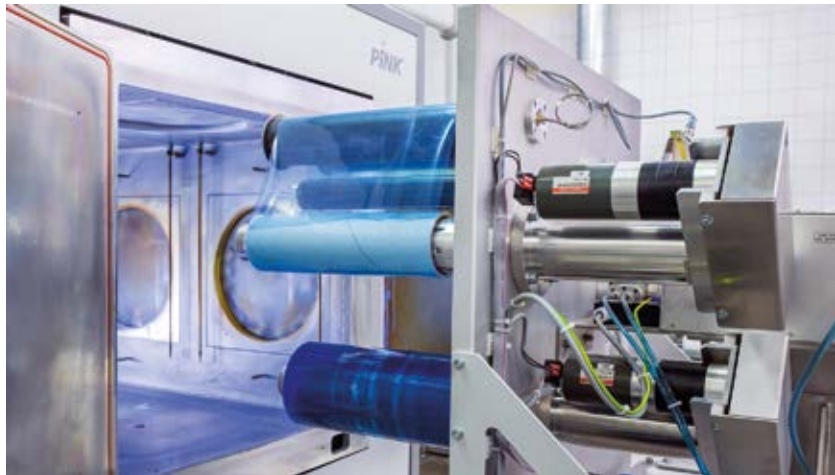
FIGURE 1: Pink V340-GKM plasma chamber for R2R coating.
